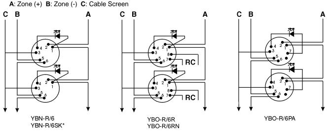
RC Relay Contacts - a flying lead on either terminal 7 or 8 selects either N/C or N/O (supplied as N/C)
